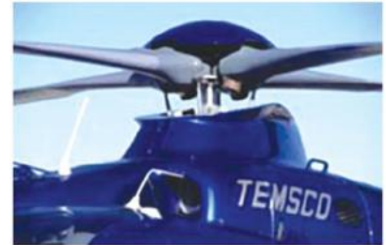
Figure 3-85. Eurocopter Model 135 rigid rotor system.
