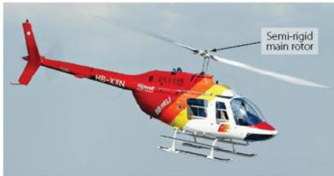
Figure 3-84. Bell Jet Ranger with semi-rigid main rotor.
